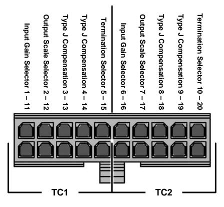
Figure 2-8: Thermocouple Configuration Jumper (JP5) Pin-Outs
